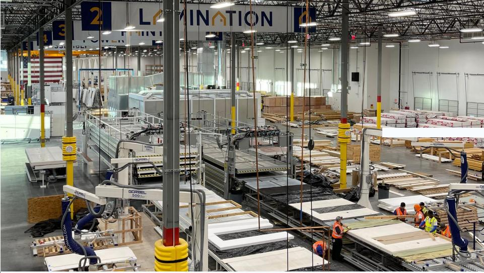
In the BOXABL factory everything is put together in an assembly line. Each station installs a different aspect of the Casita.
